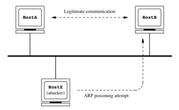
Figure 1: An ARP poisoning attack on a switched LAN
